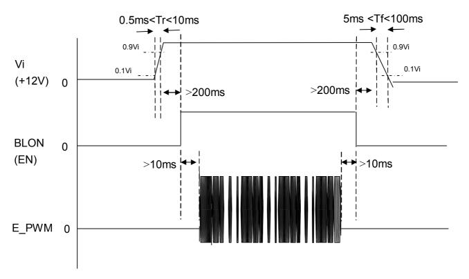
Note : While system is turned ON or OFF, the power sequences must follow as below descriptions Turn ON sequence: Vi(+12V)  $\rightarrow$  BLON  $\rightarrow$  E\_PWM signal Turn OFF sequence: E\_PWM signal  $\rightarrow$  BLON  $\rightarrow$  Vi(+12V)
